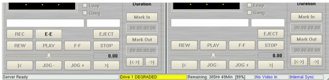
Figure 33 – GUI Drive Fault Indication
