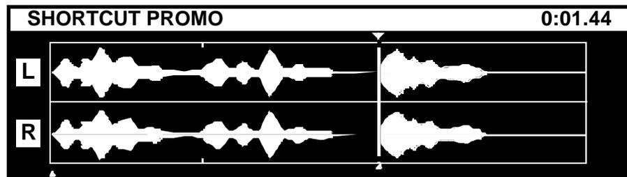
AUDIO WAVEFORM AFTER A "CUT" OPERATION
