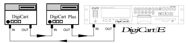
To set ECHO DURING RECEIVE on a DigiCart/E select DNET FILE TRANSFER from the Utility menu. Rotate the selection knob to set ECHO DURING RECEIVE to ON or OFF.
